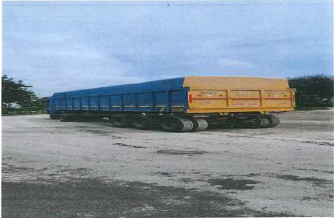
Ref 1: Transportation of Crushed material through trailer with closed body steel top
